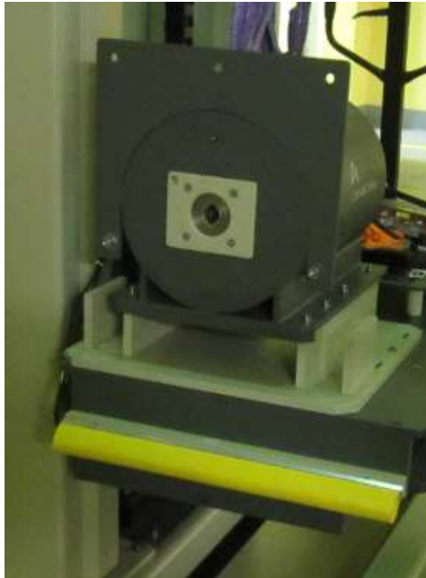
Figure 2. Close-up of the 2.54 cm TGS collimator used in the TGS system during installation.
